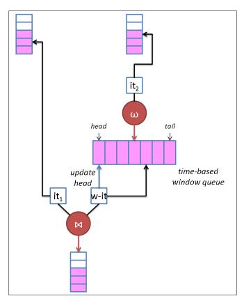
Figure 4.4 – Window-join schema
