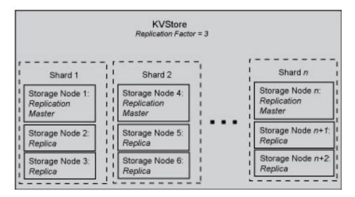
Note that if the machine hosting the master should fail in any way, then the master automatically fails over to one of the other nodes in the shard. (That is, one of the replica nodes is automatically promoted to master.)
