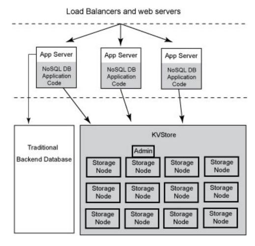
Every Storage Node hosts one or more Replication Nodes, which in turn contain one or more partitions. Also, each Storage Node contains monitoring software that ensures the Replication Nodes which it hosts are running and are otherwise healthy.
